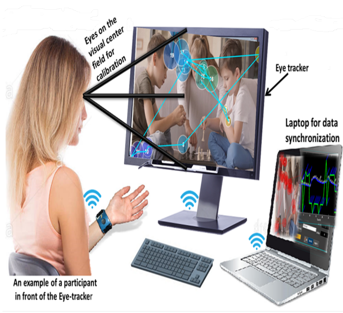
Figure 2: An example of a user interacting with video content inside an eye-tracker, a laptop for wireless data synchronisation and analysis.
